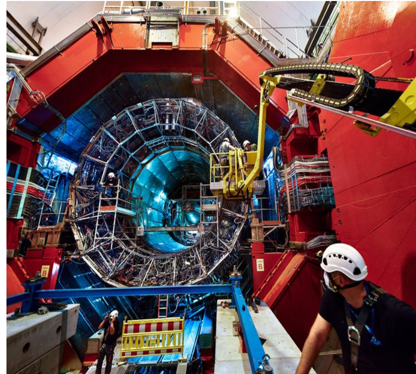
ITS and TPC removed installation of upgraded detectors TPC and (new) ITS2 March 25, 2021
